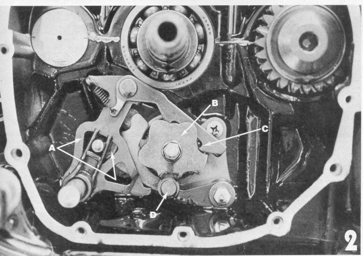
The arrows (A) indicate the areas of the shift-spindle window that must be ground away so that the shift-drum cam (B) will be pushed, or pulled, by the shift pawl (C) into correct position over the shift-drum centering roller (D).
