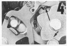
drum that engage similar tabs of the shift spindle if the drum continues past its correct position. It is possible that the end of the tab on the shift spindle will contact the shift drum before you are finished grinding the window. If this occurs, remove small amounts of material from the end of the tab on the spindle so that it will not rub on the drum and interfere with shifting.
