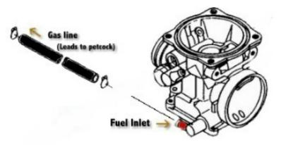
Going a little farther, Stage I: Shut off fuel petcock. Drain carburetor into container. Remove fuel line at carburetor input. Insert carburetor cleaner spray can nozzle into carburetor fuel inlet port. Spray the Dickens out of that sucker, until pure carb cleaner flows into container. Reconnect the fuel line and cycle the float bowl with gasoline as before; shut the drain screw and giver 'er a try.
