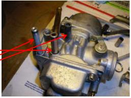
carb 2 to carb 1's tubes. Twist the accel pump and fuel "T" as you press the carbs together so you get a firm seating of the O-rings in their ports. Make sure carb's sync tab is over the top of carb 2's.
