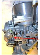
We'll use that bent paperclip again here, as we set up the spring to receive the right half bank. Turn the 1 / 2 half bank on its carb #1 side. Use your thumb and forefinger to turn the spring counterclockwise to get that horizontal hook onto the choke actuator tab. The vertical hook will be barely showing just above or below the shaft tabs – you may have to twist the spring counterclockwise to get the vertical hook to show itself BELOW the tab.
