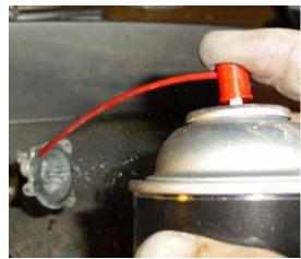
Sometimes you can soak just the check-valve, by setting the cap right side up in the spray-can cap, and fill it with carb spray. Let it sit for an hour or so, and try again. Run spray through each jet and emulsion tube, paying special attention to the aeration holes on the sides (make sure they're clear).
