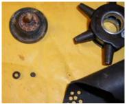
Place the rubber "plug" you just cut <u>under</u> the O-ring on the body. I use some pretty thick rubber, so it fits inside the O-ring and stays put. Some folks prefer thinner material and put it between the O-ring and the body of the carb – whatever way, you want to block off the angled vacuum port coming from the inside of the carb throat. Now just reinstall everything; make sure to install
