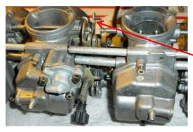
OK, one last tricky part (here's where I usually swear like a sailor). As you connect the two halves together, be careful not to bump the vertical hook of the choke spring off of its perch on the vertical tab of the choke shaft. You want to loosely insert the left sides of the vent tube, fuel tube and accel tube into/onto their respective ports of carb 2, but watch carefully as the tines from the 3 / 4 choke shaft get close to the choke spring. When it's right up against the spring, take either
