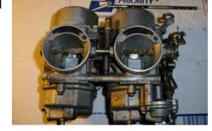
the 4 choke screws, carefully remove the choke shaft and choke spring (it will be hooked to the main choke arm).
