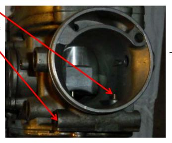
body side of the nozzle. You can use your needle-nose pliers to hold the E-string and blindly search for the hole – once you've found it, wiggle the string in there, and try again. You may have to soak the carb body and run it through the ultrasonic cleaner again to clear this nozzle.
