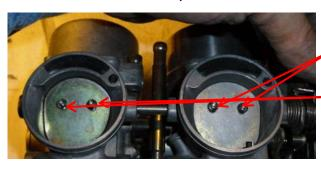
so the choke plate reliefs are pointed towards you. Place a choke plate on #2's relief and loosely install two 3mm x .5 x 6mm screws. Snug them up and back them off 1 full turn. Repeat for carb #1.
