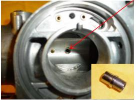
secondary main jet emulsion tube, and MAY fall out when you remove the tube. If so, put it in the small parts tray as well.
