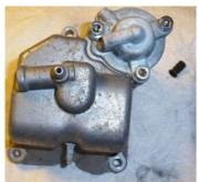
Carb #2 is special in a number of ways, as you've already seen. The last special thing we'll work with is the accelerator pump — a small diaphragm, spring and set of special check-valves that squirt fuel directly into the throat of each carb when the throttle is twisted briskly. This is meant to overcome the "turbo-lag" of the heavy vacuum needle pucks that make these CV carbs so unique.
