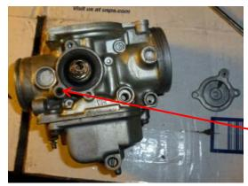
Carefully remove the 2 screws holding the air cutoff cover while holding the cover down (there's a strong spring under the cover). Before putting the cover and the spring in the small parts tray, inspect the cover and
