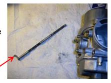
has a notch in it). Twist the shaft so the reliefs cut into the shaft are facing you (slightly facing down) and install a choke plate on each relief, and install new 3mm x .5 x 6mm screws into the choke shaft tighten them down, then back them off 1 full turn – we'll cinch 'em down later in the build. Make sure the choke shaft can turn 90° easily – if it binds, you may have to recheck that the tubes are fully seated in their ports.
