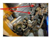
the tines fit under the throttle actuator arm. and the round hook of the spring should fit over
