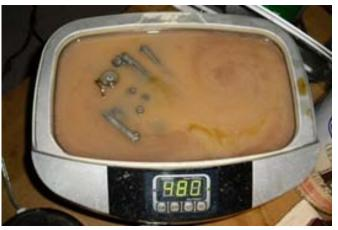
I place the carb body face down in the basket and lower it into the Dip, then (after removing the float-bowl gasket) position the other 3 major pieces around it so they're all covered in the thick liquid. Let it sit in there anywhere from 15 minutes to overnight depending on how nasty your parts are. Usually 30 minutes is plenty. Remove the parts and put in the ultrasonic – I use Pine-Sol® as the liquid for the ultrasonic. I run 'em for 15 to 20 minutes, then put them in
