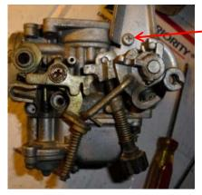
Remove the throttle cable mount (held in place by a 4mm
