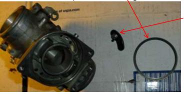
plastic air jet cover. Put the springs, sealrings and air jet covers (with screws) in the small parts tray.
