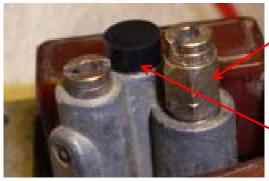
Install the secondary main jet emulsion tube (this will hold the needle jet in). Now, if you removed the slow-speed jet, install it now and put in a fresh rubber passage plug – make sure it fits snugly and doesn't fall out when you turn
