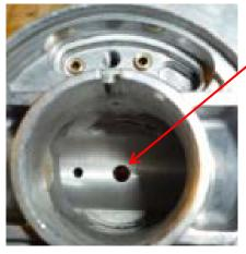
the needlejet came out with the needlejet holder (back on step 2 middle of page 12), you won't see it in the carb throat – we'll install it later on – don't worry.
