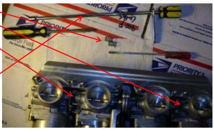
screw so its throttle butterfly matches (as closely as you can eyeball it) to carb #2's butterfly (carb 2 is the base carb, and it isn't adjusted – the other 3 are adjusted to it). Now un-wedge the throttle and let 'em close. Turn the high idle knob (black knob under and below carbs 2 & 3) in until all 4 butterflies are uncovering at least 1
