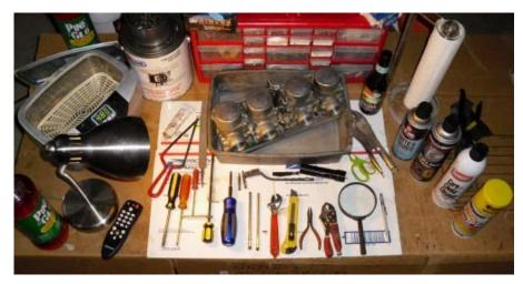
just a large coffee table covered with thick cardboard. You need to have enough room to set up your tools, layout the parts of the carbs and a cleaning area to clean the parts. You'll want a plastic pan such as those used for oil changes for cleaning the individual parts prior to assembly. It should be impervious to the chemicals used in spray carb-cleaner or brake-cleaner.
