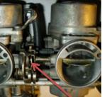
Turn the carbs on their tops and remove the eight 6mm screws from the front rail (you may need a
