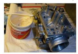
Without a doubt, the second most important thing about your carb cleaning process (right after the slow-speed jet and passage cleanliness) is the float valve seats. More people complain about their carbs pissing fuel out the overflow tubes, and it's almost always caused by dirty float valve seats. Get yourself
