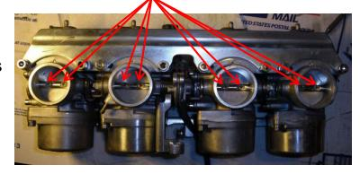
open position. If they don't, they're binding because they're not aligned properly and should be re-adjusted. Once they do that, go ahead and tighten up those 8 throttle butterfly screws nice and snug (don't strip the screw head – use a big bit here).
