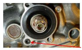
Take the air cutoff cover, place the conical tip of the straw into the hole in the corner and spray you should get a jet out the side hole just beside it. If you got new diaphragm kits, install the diaphragm (make sure the brass tip easily slides into the hole, and the diaphragm lip fits securely in the groove). Place the rubber O-ring in the hole in the lower left corner of the air cutoff hole in the
