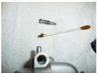
Use the carb cleaner spray and the acid brushes to clean out any residual gunk in the bottom of the float bowl. Use a Q-Tip® to clean out the seat of the float bowl drain screw. Start with a full tip, and then pull off enough of the cotton off the end of the Q-Tip® to go all the way through into the base of the float bowl. Trust me; they'll be black with goo – keep using the Q-Tips® and carb spray until they are clean.
