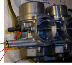
Now, install the long fuel tube (unless these are 1000 or 1100 carbs), and the long accel pump tube, as well as the vent "T" on carb #3/ in preparation for bringing the two halves together.
