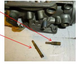
slot and don't force it. These get corroded in sometimes and you can do more damage to the thing by stripping out the screw slot. If it's stuck in there, try spraying some PB-Blaster down the hole and let it sit overnight. Worse case, you can clean
