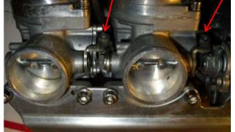
bottom up and being careful to not crossthread the screws. Once the screws are in, go ahead and install the locknuts finger-tight. Now it's time to bench-sync the carbs. This gets the throttle butterflies open an equal amount so then final syncing on the running motorcycle will be quicker. Often, if the engine valves are already adjusted to their .004"-.006" specs, the carbs will bolt on and run with no significant touchup required!
