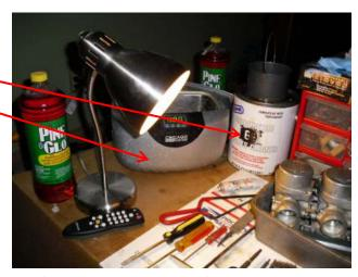
clean off nearly all your caked on oil and grime from the outside of the carb, as well as the varnished gasoline throughout all internal surfaces of the carb bodies. Now others will swear by a simple 2-gallon pail, and a gallon of Pine-Sol®. It's up to you – both methods work well.
