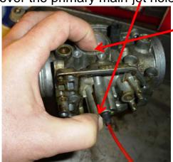
over the lower air cutoff hole and spray. If the slow-speed jet is truly clear, you'll get a bubbling (or stream) of carb spray out the pilot screw hole. Don't consider the carb cleaned until you can do that!
