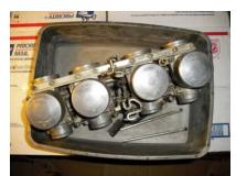
Remove all hoses from the bowls and any fuel lines from the carbs. If your bike has the vacuum-assisted petcock on it (AKA Spawn of Satan or SOS), remove it, but keep all the tubes connected to it.
